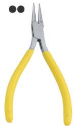
J-803 Round Nose Pliers 120mm Carbon Steel Made Nickle Plated, Box Joint Pvc Handles.
