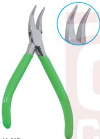
LL-807 Chain Nose Pliers Curved 115mm Stainless Steel Made, Box Joint with Double Leaf Spring, Satin Finish Pvc Handles.
