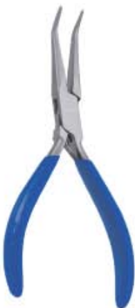
J-980 Long Chain Nose Pliers Bent 150mm, with Single Leaf Spring Stainless Steel Made, Pvc Handles.
