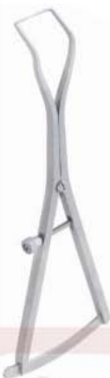
DE-1815 Measuring loop, Castroviejo angled, length 175 mm, measuring range 0 - 40 mm, with window
